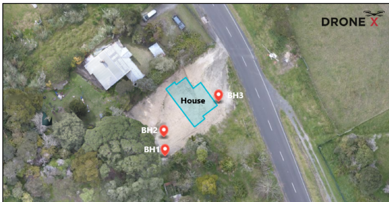
Figure 8 - Borehole Location Overview (adapted from DroneX aerial survey.)
