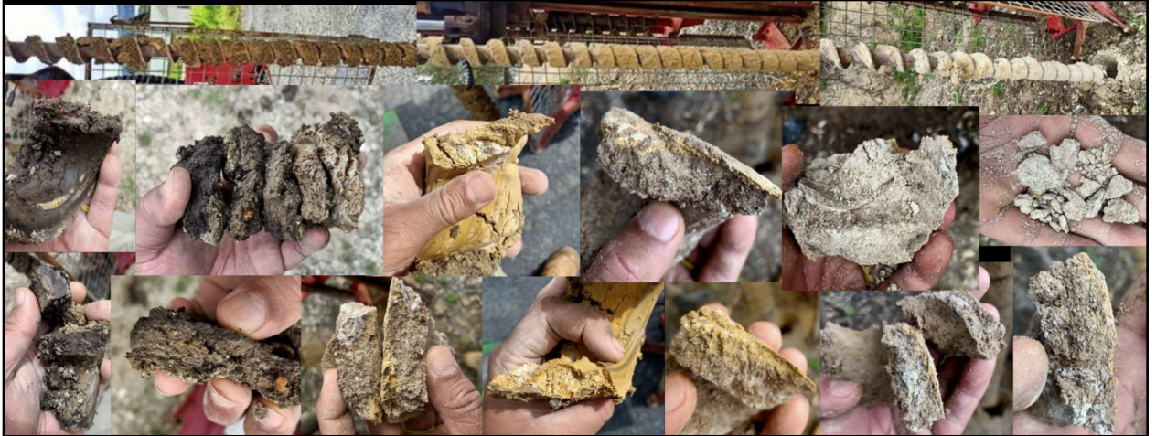
Figure 9 - Natural Soils Onsite - BH1 borings (adapted from the DroneX Survey).
