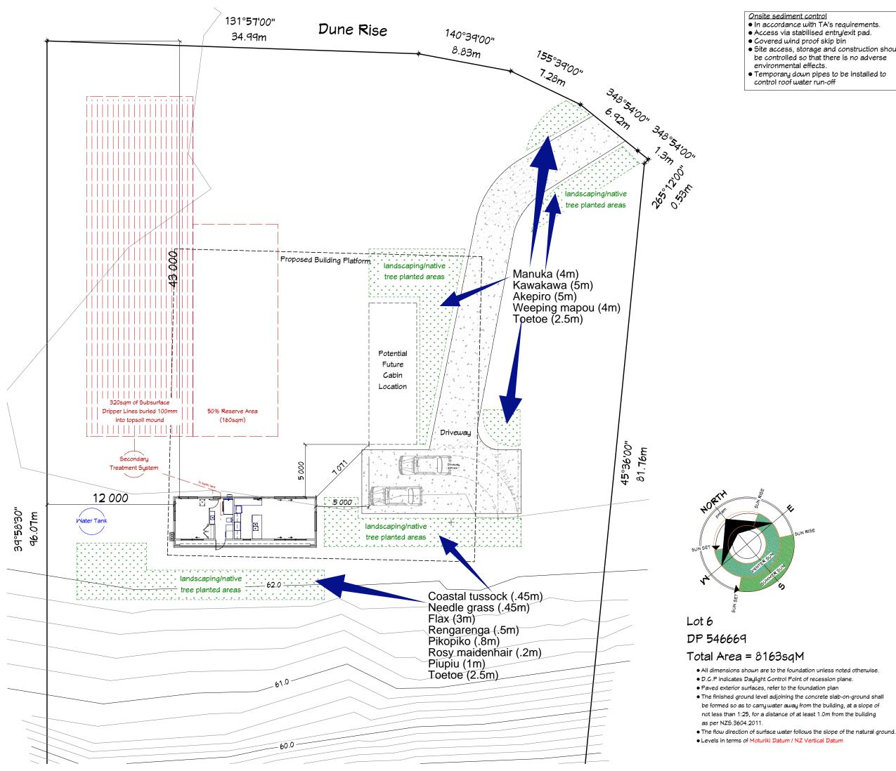
In accordance with TA's requirements. • Access via stabilised entru/exit pad. • Covered wind proof skip bin • Site access, storage and construction should be controlled so that there is no adverse environmental effects. • Temporary down pipes to be installed to control roof water run-off
