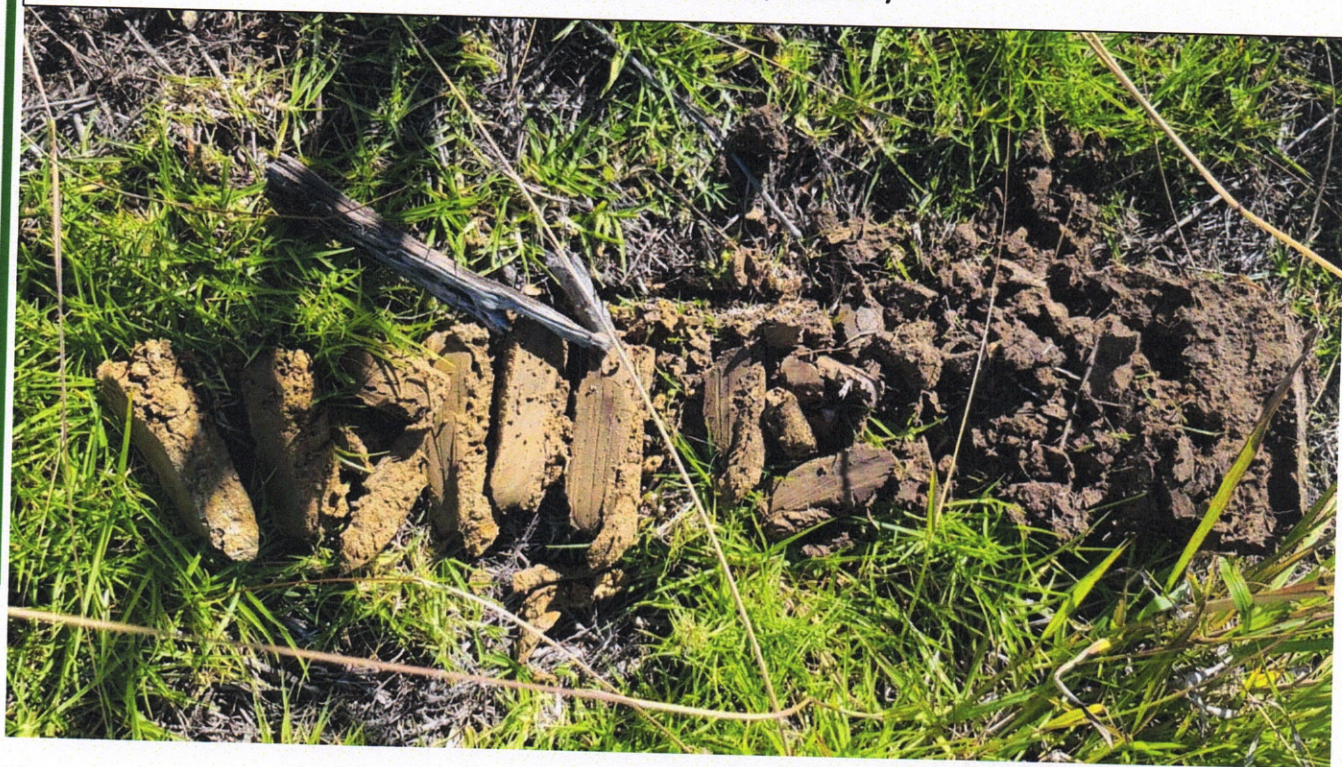
Soil Profile: 250mm Loamy Topsoil over Sandy Clay Loam Class 5, (as per AC TP-58, Table 5.1)
