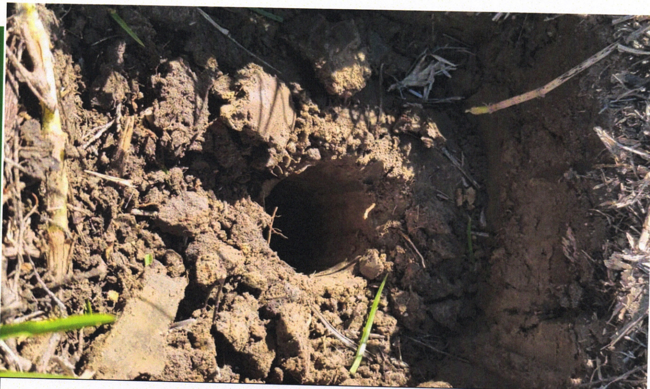
Soil Profile: 250mm Loamy Topsoil over Sandy Clay Loam Class 5, (as per AC TP-58, Table 5.1)
