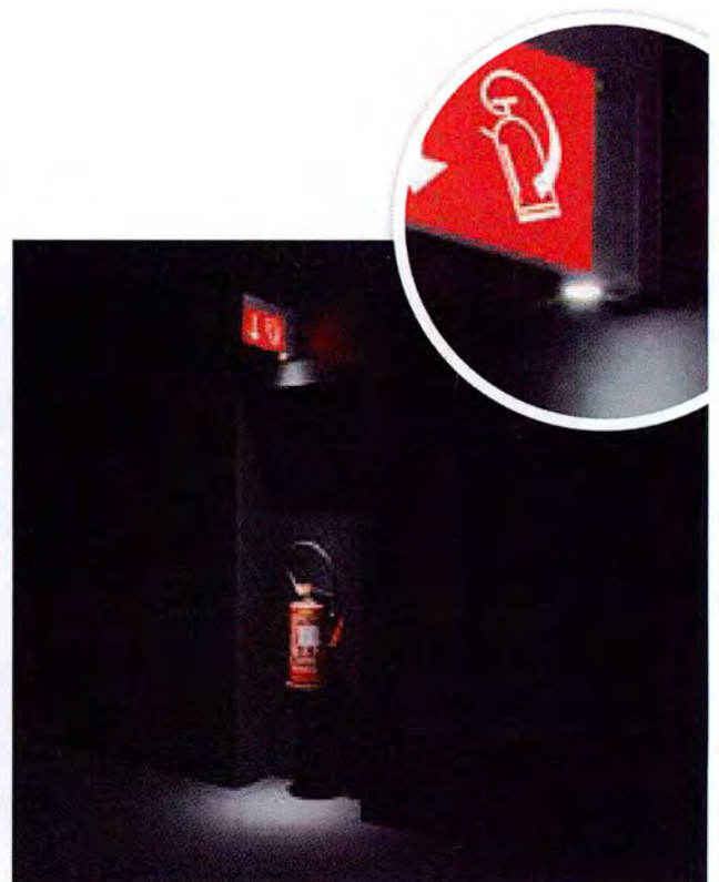
With a light spot module 5 lux is achieved, up to 4 metres mounting height without extra luminaires.
