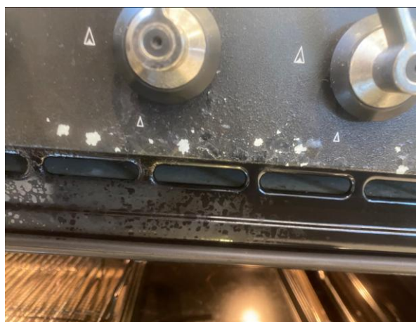
Heat damage to surface above top of oven door
